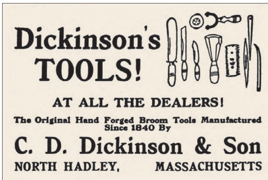
Advertisement showing broom making tools including knives for cutting and trimming tassels and needles used to stitch the brooms. From Brooms, Brushes and Handles , 1919.
